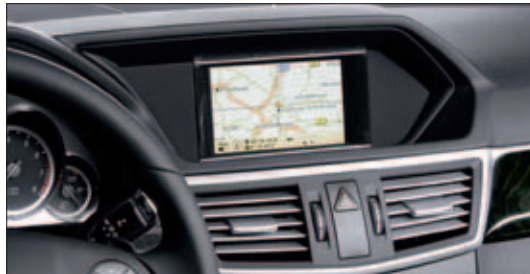
Central display unit with 5.8-inch screen
