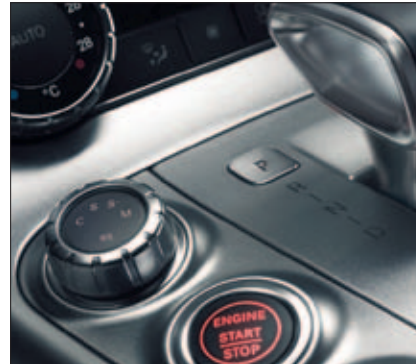
The AMG Drive Unit with AMG E-Select gear shift lever and Keyless-Go start function
